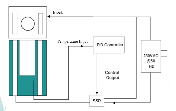
As Shown in above diagram, SS block is heated in such a way that a cavity in block has radial as well as axial homogeneous temperature. This temperature is sensed by highly accurate and stable sensor and block temperature is controlled by a PID controller.
