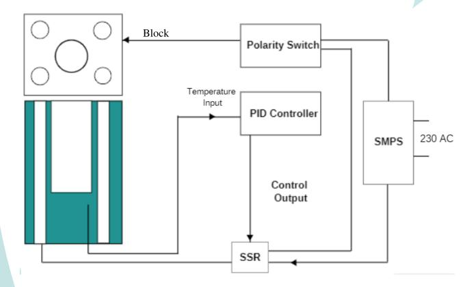
As Shown in above diagram, Aluminum block is heated & cooled by Thermoelectric coolers in such a way that a cavity in block has radial as well as axial homogeneous temperature. This temperature is sensed by highly accurate and stable sensor and block temperature is controlled by a PID controller.
